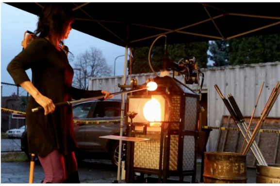
5 of 11 | Molten glass leaves the furnace at more than 2,100 degrees Fahrenheit. The glowing piece at the end of the rod is called a "gather." (Alan Berner / The Seattle Times)
